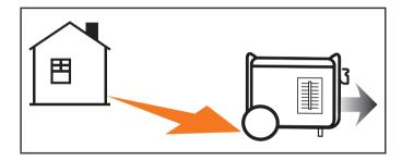
If misused and operated in an unapproved and unsafe location that results in the accumulation of poisonous CO gas inside an enclosed or partially enclosed space, for example a house, garage or a garage with the door partially open, CO Shield® will automatically shut off the generator and then will illuminate a blinking red LED light. **Read the action label for next steps.**
