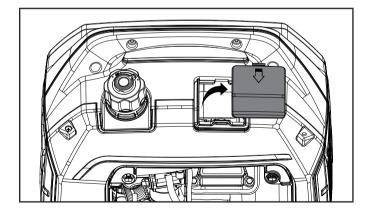
3. Remove the spark plug cable from the spark plug.
