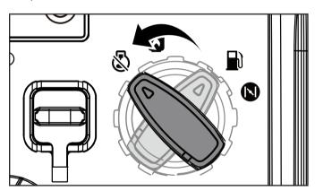
**Important:** Always ensure that the dial and fuel vent on the fuel cap are in the "OFF" position when the generator is not in use.
