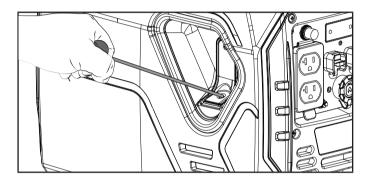
6. As the engine warms up, turn the EZ Start dial to the "GASOLINE OPERATION" position.
