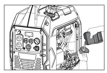
5. Check engine oil level before each use and add as needed.
