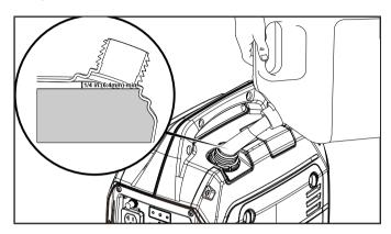
3. Screw on the gasoline cap and wipe away any spilled fuel.
